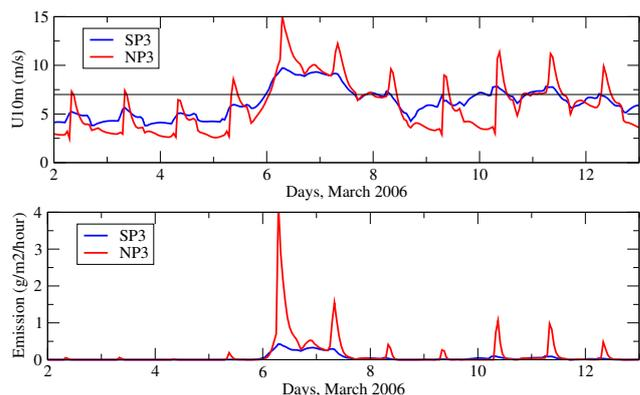
**Figure 3.** Comparison from 2 to 13 March 2006 of the  $10 \text{ m}$  wind (upper panel,  $\text{m s}^{-1}$ ) and emissions (lower panel,  $\text{g m}^{-2} \text{h}^{-1}$ ) for simulations SP3 (blue) and NP3 (red) in the grid cell, selected for emission analysis at  $7.5^\circ$  W,  $18.5^\circ$  N (shown in red in Fig. 1). The horizontal line in the upper panel corresponds to a wind of  $7 \text{ m s}^{-1}$ , above which emissions start to be significant.
