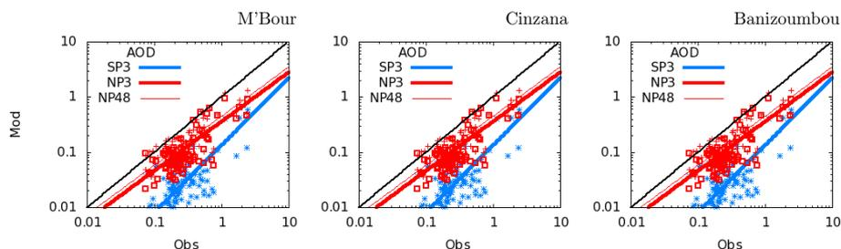
**Figure 6.** Scatter plots of the model vs. observed AOD at M'bour, Cinzana and Banizoumbou for simulations SP3 (blue), NP3 (thick red line and squares) and NP48 (thin red line and crosses) computed at daily frequency.
