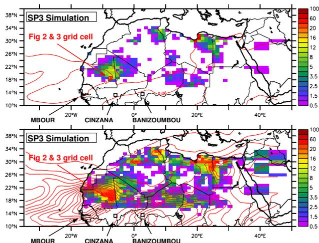
**Figure 1.** Comparison of the total emission ( $\mu\text{g m}^{-2} \text{s}^{-1}$ ) for the SP3 (top) and NP3 (bottom) simulations (NP and SP versions of the physical package with  $\tau = 3$  h for nudging) for March 2006. Contours correspond to the mean AOD at 550 nm, with a 0.02 interval between contours.
