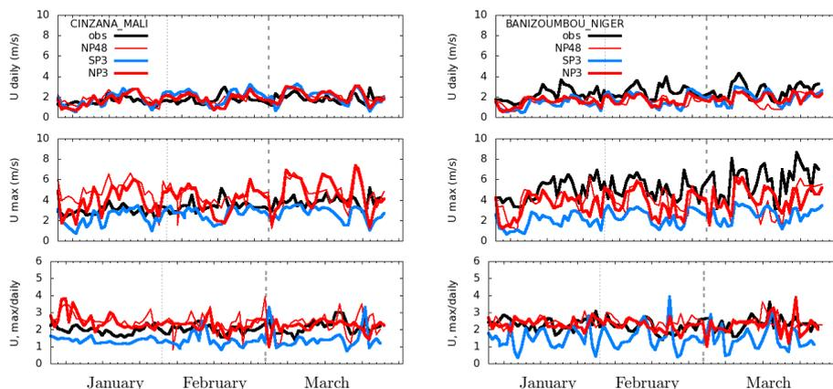
**Figure 4.** Time evolution over winter 2006 of the daily mean (upper panels) and maximum (middle panels) 10 m wind speed ( $\text{m s}^{-1}$ ) as well as the ratio (lower panels) of the maximum value to the daily mean for Cinzana (left) and Banizoumbou (right). Results of the SP3 (blue), NP3 (thick red line) and NP48 (thin red line) simulations are compared to site observations (black).
